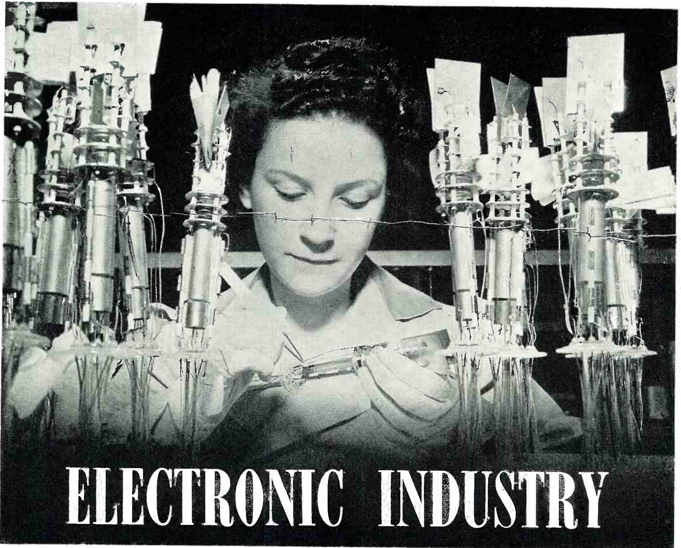
Checking mount mechanism of cathode-ray tubes in an air-conditioned, dustless room.
