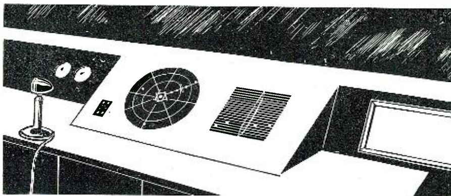
Fig. 8. Scanning screens installed in airport traffic control towers.
