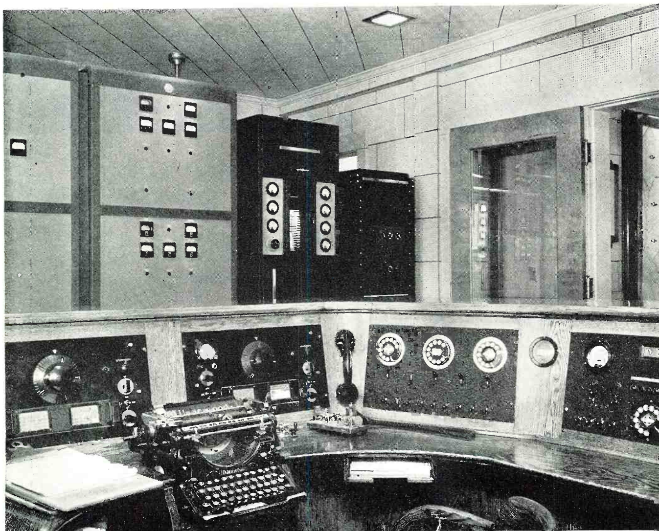
Radio operator's position at the control panels of the Buffalo Police Department radio station.
