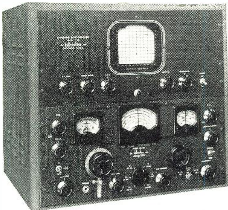
The S-35 panoramic adapter and SX-28 communications receiver mounted as a unit.
