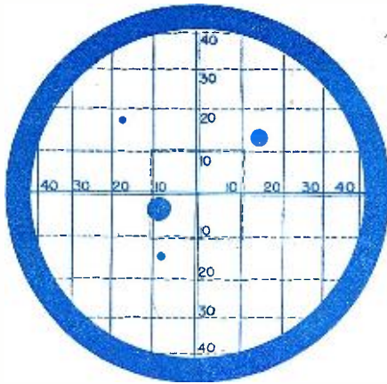
Fig. 4. Horizontal separation indicator. Dots indicate position of other planes.
