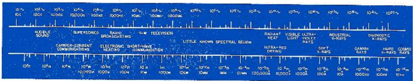
Fig. 1. The electro-magnetic spectrum covering a frequency range from 10 to 10^{20} cycles. The unit XU is equal to 10^{-11} cm.
